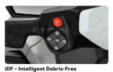
**Pump System** An innovative, industry-first system that allows you to free your pump of weeds and debris with intuitive handlebar-activated controls.
