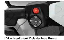
System (Optional) An innovative, industry-first system that allows you to free your pump of weeds and debris with intuitive handlebar-activated controls.
