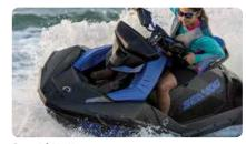
Spark® Hull The Spark hull design provides a lightweight and playful platform. The innovative Polytec<sup>™</sup> material further reduces weight while optimizing performance and efficiency. The color-in molding is more scratch-resistant than fiberglass.
